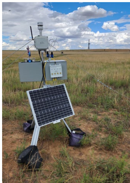
A detector stationed near a well pad in Colorado's Denver-Julesburg Basin is monitoring air quality during drilling operations as part of a study led by Jeffrey Collett of Colorado State University.
